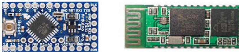
Fig. 6. The MCU module: Arduino Pro Mini (left) together with the Bluetooth module: HC-06 (right).
