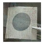
**Fig. 3.** Photographic image of Cs<sub>3</sub>Sb photocathode in a circular shape formed on the microstructure.
