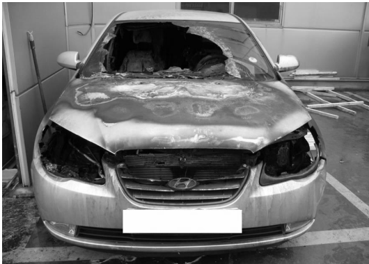
Fig. 4. Fire example by overheating of heat wires heating seat.
