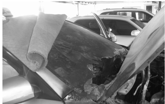
Fig. 2. Fire example by air freshener explosion putting on crash pad of a car.
