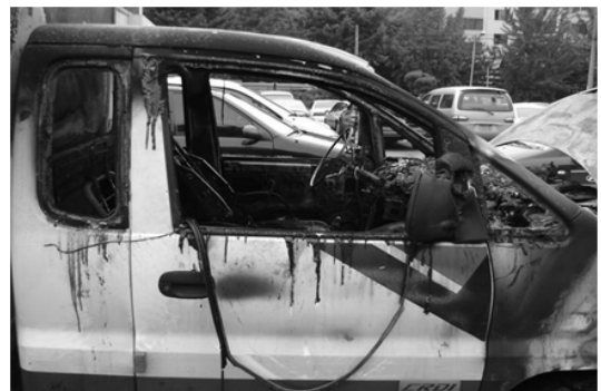
Fig. 3. Fire example by overload of electric power part in a car.
