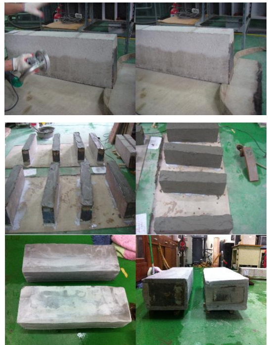
[Fig. 2] Surface treatment and strengthening by DFRCC
