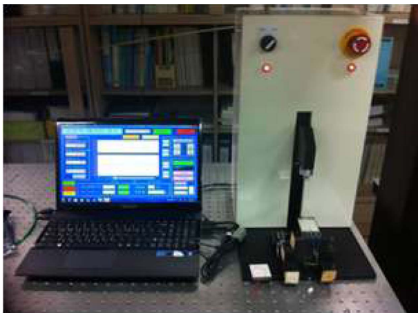
Fig. 5. Test setup of the displacement applying system.
