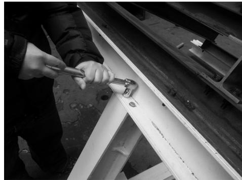
Fig. 7. Torque Wrench and Torque Release Measurement
