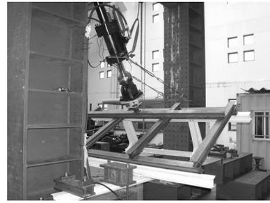
Fig. 5. Dynamic Test Specimen of Floating PV Generation Structure
