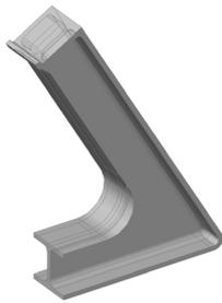
Fig. 14. Vertical Member Made by SMC Process (Choi et al., 2013)
