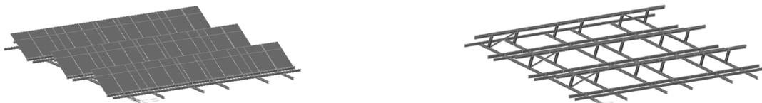
Fig. 3. FE Analysis Model of Floating PV Generation Structure
