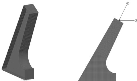
Fig. 16. FE Analysis Model of SMC FRP Vertical Member
