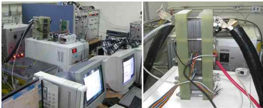
Figure 5: Stack activation Test
