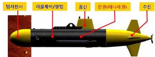
Figure 1: Structure of a typical UUV
