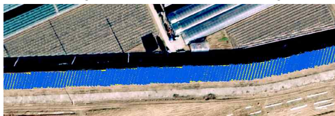
(b) LiDAR points(blue dots) located in the levee top polygon
