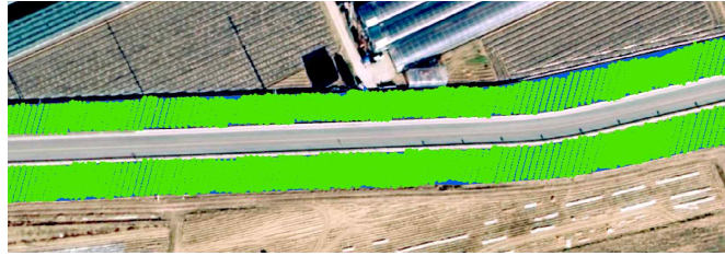
(c) LiDAR points(green dots) located in the levee slope polygons
