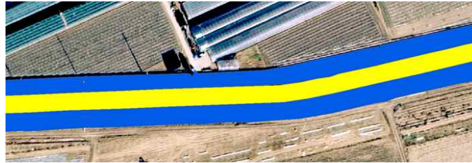
(b) Levee crown polygon(yellow polygon) and levee slope polygons(blue polygons)
