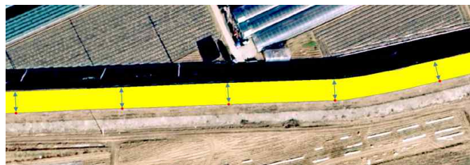
(a) Checkpoints(red dots) generated at 50 m interval along the levee top polygon
