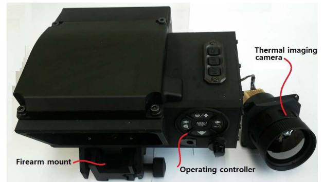
Fig. 9. Fabricated configuration for the new designed day & night scope with a BS prism.
