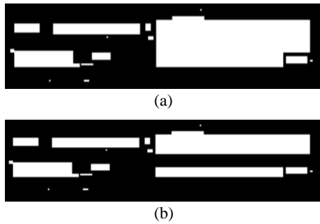
Fig. 4. Process of dividing big blob Rectangle (a) input (b) divided big blob
