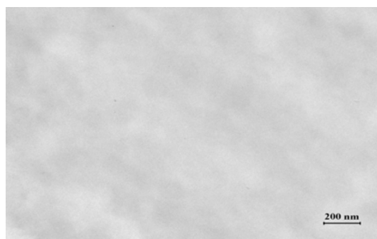
Fig. 2. A TEM micrograph of the pure rubber latex.
