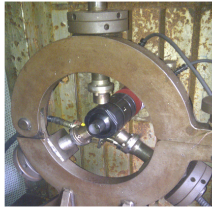
Fig. 5 Static firing test of dual-thrust flight motor for performance evaluation.
