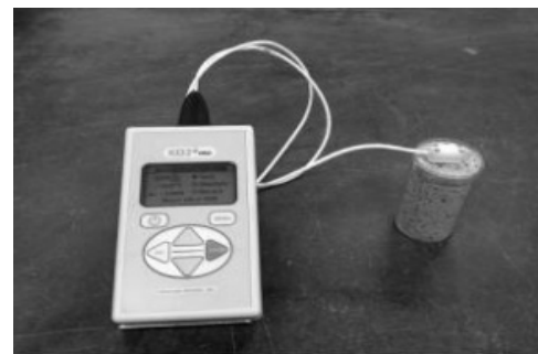
Fig. 4. Thermal conductivity test apparatus (K-D2-P)
