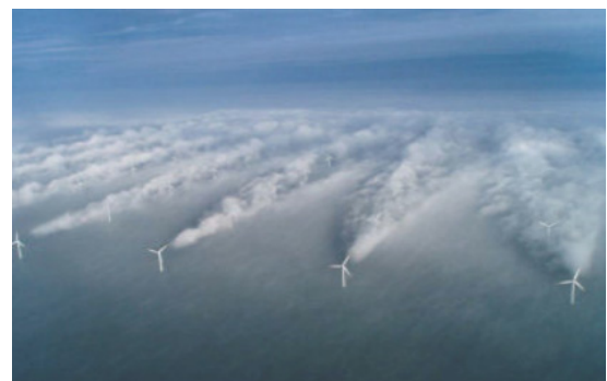
Fig. 1 Wake effect in Horns Rev. wind farm(owned by Vattenfall. Phothographer Christian Steiness)
