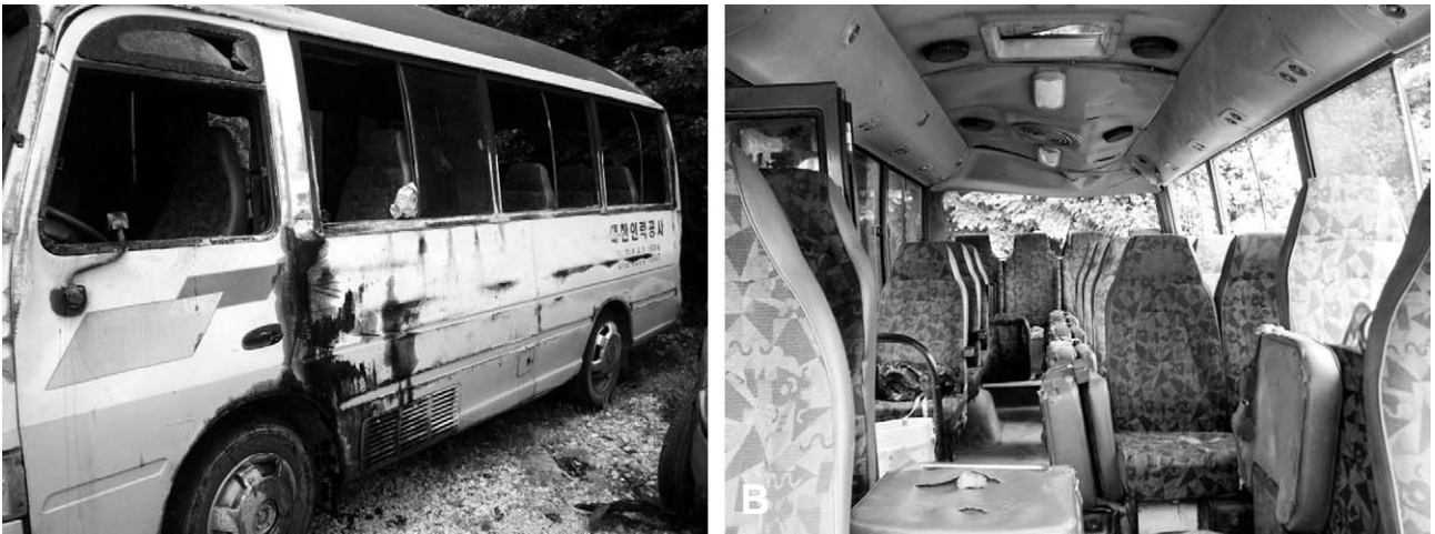
Fig. 2. Exterior and interior photo of a 25-passenger bus. ((A) left side of vehicle, the scratches and broken windows shows the evidence of one quarter turn rollover accident. (B) the site of roof collapse lies at the rear of the bus cage)
