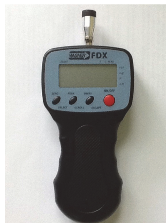
Fig. 1. Pressure algometer(WAGNER FDX)
