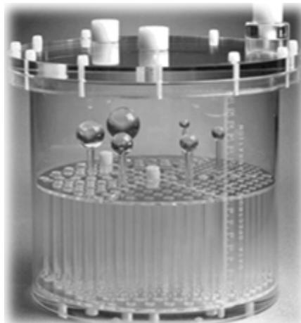
Fig. 2. ACR Phantom was used for this study.
