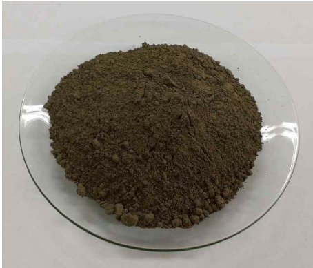
Fig. 1. Crushed Mn nodule slag sample generated by smelting reduction process.
