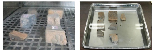
(a) Measure of weight after dry ( m_1 ) (b) Measure of weight after submerge ( m_2 )
