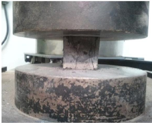
Figure 4. Measuring method for compressive strength.
