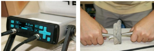
(a) Measuring equipment (b) Measuring method Figure 3. Equipment and method for ultrasonic wave velocity measuring.
