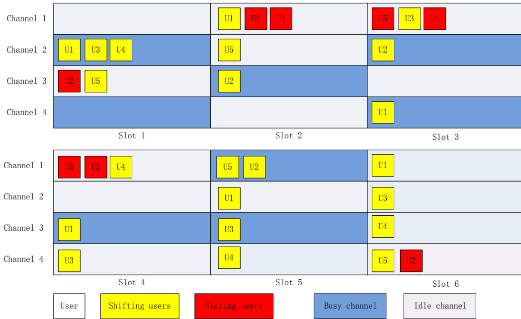
Fig. 2. An example to illustrate the convergence (Slot 1-5 are the convergence process and Slot 5-6 are both the "convergence" state).
