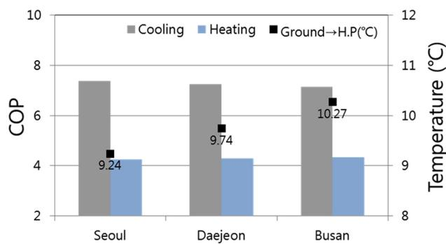
Fig. 11. Heat Pump COP of Heating and Cooling
