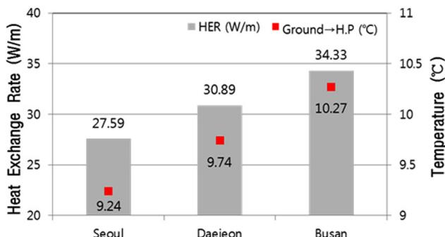
Fig. 8. Heat Exchange Rate and Heat Source Temperature in Heating
