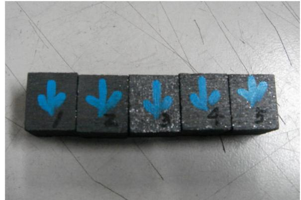
**Fig. 1** Specimen for compressive strength
