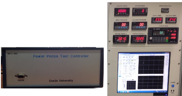
(c) test controller and console
