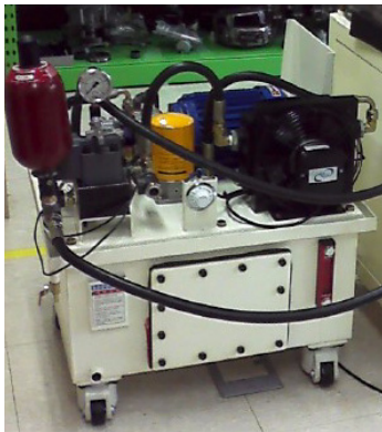
(a) hydraulic power unit
