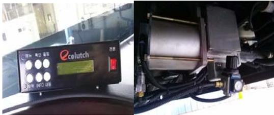
[Fig. 12] Photo of Semi-automatic clutch controller on dashboard and pneumatic actuator on frame
