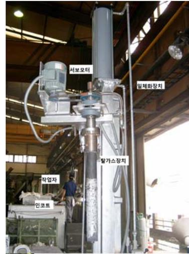
[Fig. 2] Degassing device configuration
