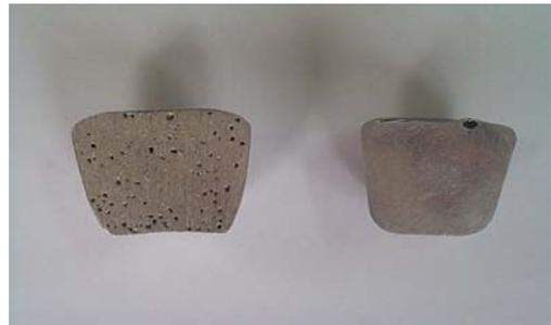
[Fig. 7] Degassing operations before and after the pore inspection
