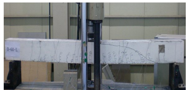
Fig. 3 Typical shear failure
