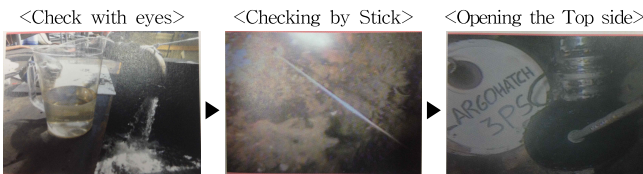
Fig. 6 The pictures of checking the recovery work termination on M/T Kyung-Shin
