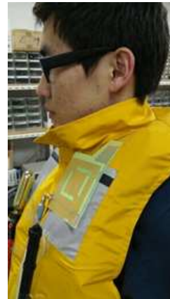
Fig. 10. Configuration of antenna integrated into lifejacket
