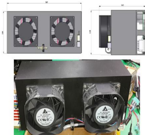
Fig 5. A Ultra-light Fuel Cell System Part of 600 W fuel cell system developed by DGIST
