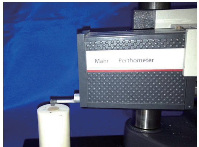
Fig. 4. Perthometer M2 (Mahr GmbH, Göttingen, Germany).
