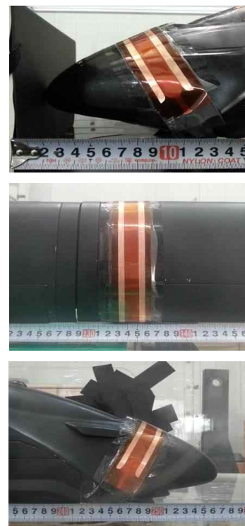
Fig. 13. SD plasma actuators which are mounted on front, middle and rear parts of the mock-up model (700 mm, 1320 mm and 2440 mm away from the train nose, respectively)
