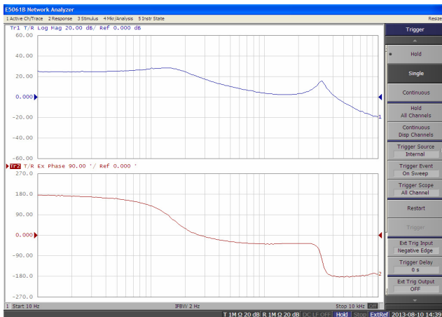
Fig. 8. Bode diagram of G_{vd}(s) from the circuit experiments
