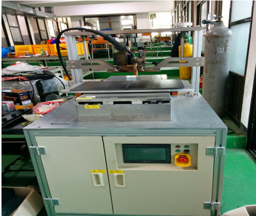
Fig. 13 Automatic welding equipment
