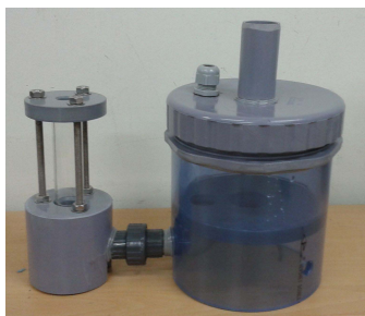
Fig. 8 Solution tank and cylinder for liquid level measurement
