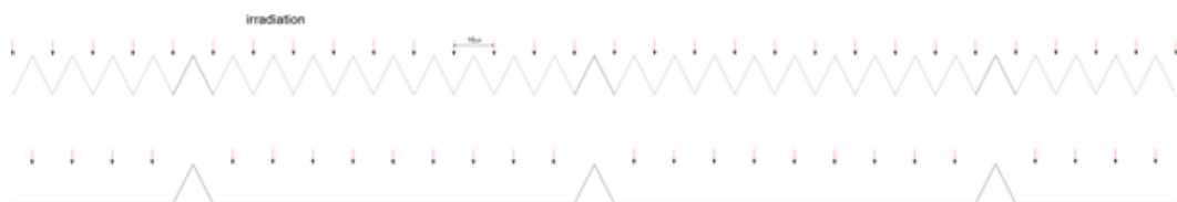
Fig. 4 Schematic of stepwise laser relief engraving.
