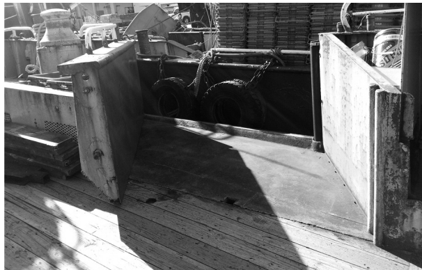
Fig. 2. A side opening for hauling net on the side trawler, Yoo Jin.
