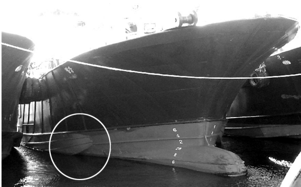
Fig. 3. The side bulge of the side trawler.
