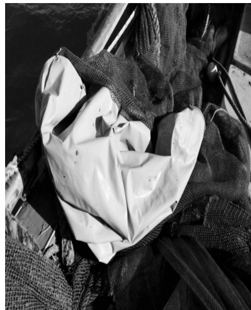
Fig. 2. The round canvas attached to the end of the cod end in the shrimp beam trawl.
