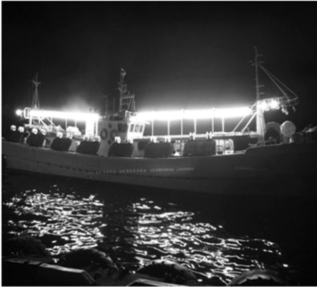
Fig. 2. Photograph of LED fishing lamps at the experimental squid jigging vessel (24tons).
