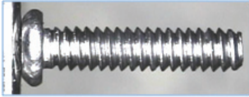
Fig. 13 Fabrication of an asymmetric screw (asymmetric angles: -20^\circ )
