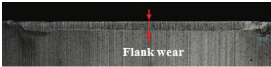
Fig. 5 Flank wear at cutting speed of 300m/min
