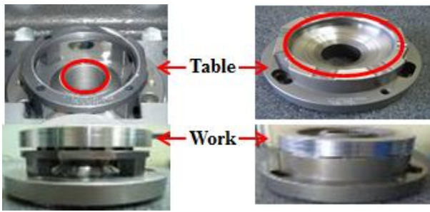
(a) Before (b) After Fig.13 Table shape of T/F driven gear in broaching process
