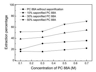
**Figure 5.** Effect of the PC 88A concentration on the extraction of K using different saponification degree from synthetic solution.
