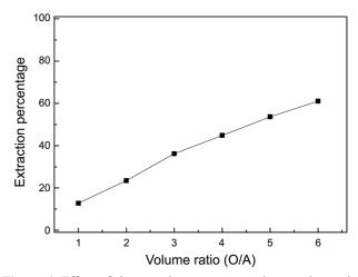
Figure 6. Effect of the organic to aqueous volume ratio on the extraction of K by 50% saponified 0.7 M PC 88A from 50 wt % molasses-water mixture.
