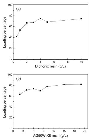
**Figure 2.** Effect of resin concentration on the adsorption of K from synthetic solution.
