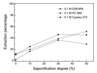
**Figure 4.** Effect of the saponification degree on the extraction of K from synthetic solution.
