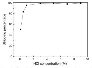
**Figure 8.** Effect of HCl concentration on the K stripping, Loaded organic was obtained by extract K from 50 wt % molasses-water mixture with 0.7 M 50% saponified PC 88A at O/A ratio of 6.
