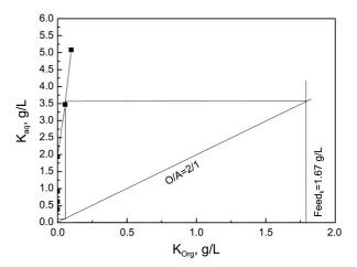
Figure 9. McCabe-Thiele plot for K stripping, Strip solution = 1 M HCl, K in loaded organic phase = 1.67/L, Loaded organic was obtained by extract K from 50 wt % molasses-water mixture with 0.7 M 50% saponified PC 88A at O/A ratio of 6.
