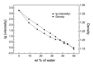
Figure 1. Effect of wt % of water in molasses on the lg (viscosity) and density at 25 °C.
