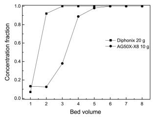
**Figure 3.** Variation in the concentration fraction of K with bed volume in the effluent during continuous experiments from 50 wt % molasses-water mixture.
