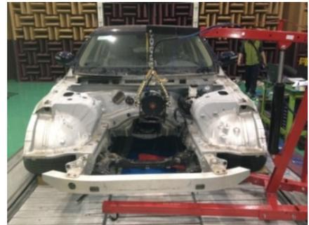
**Fig. 9** Experimental setup of trimmed body
