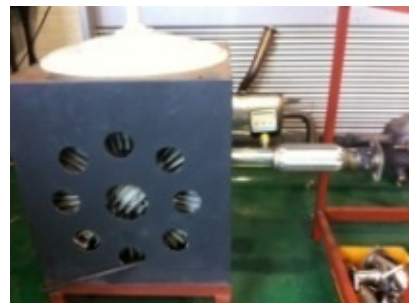
Fig. 9 Picture of test setup for back-pressure measurement, provided by Pico Corp.
