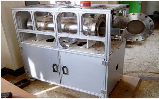
Fig. 1. Pressure treating cylinder.
