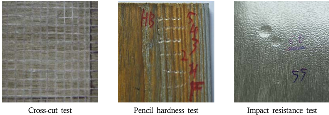
Fig. 4. Cross-cut, Pencil hardness, Impact resistance tested specimens (From left to right).
