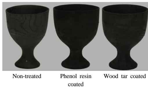
Fig. 4. Picture of non-treated and phenol resin coated wood charcoal cup carbonized at 600°C.
