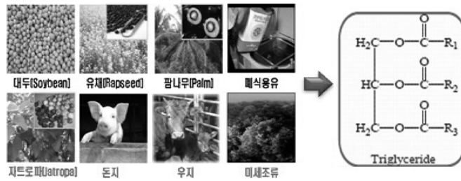
Fig. 1. The raw materials and main components Bio heavy oil.
