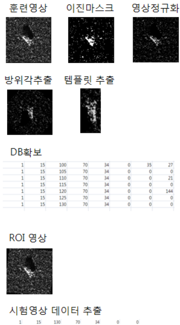
Fig. 6. Step-by-step application example of template matching based automatic target recognition algorithm
