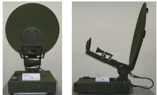
Fig. 7. The fabricated geometry of the fly-away satellite terminal
