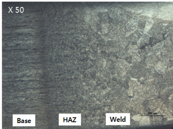
Fig. 6. Microstructure in weld metal of an electron beam welded Ti-6Al-4V
